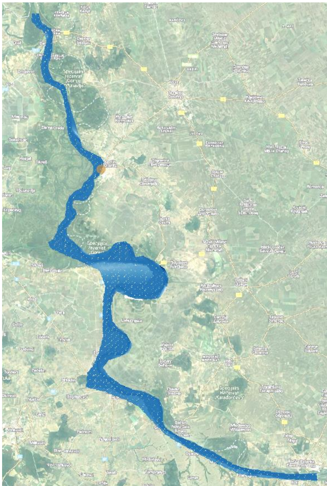
Figure 4: Geographic coverage of the LIDAR survey, showing that only the right riverbank and a portion of the Danube River were surveyed
