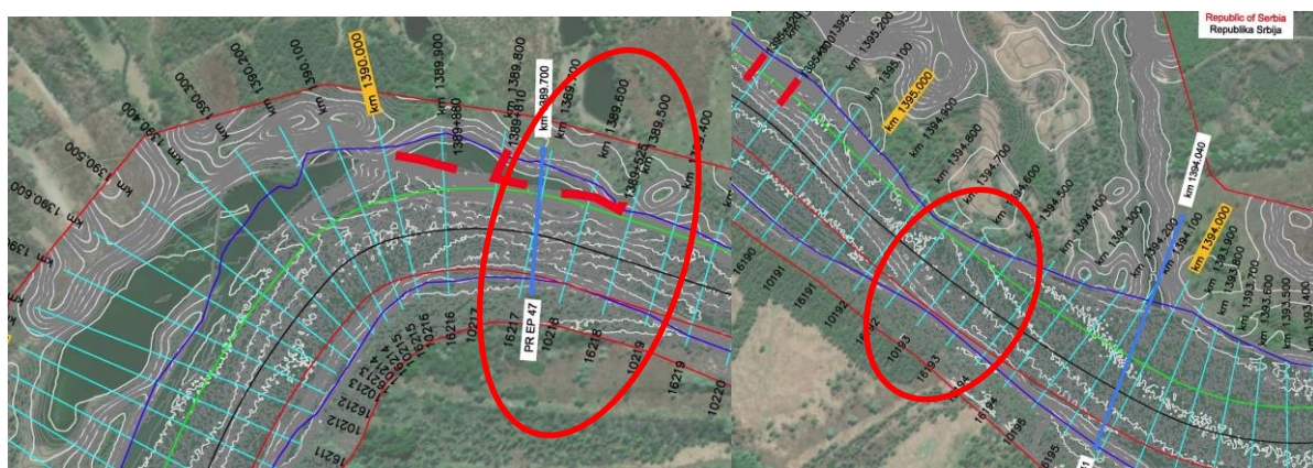
Figure 11 - The contractions in the Civutski / Zidovski rukavac sector on km 1394.6 and 1389.5
