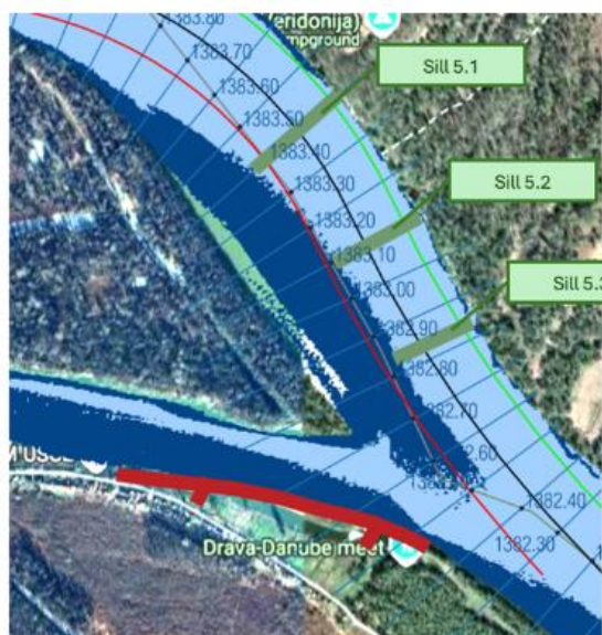
Figure 40 - Scenario 4 – overview of the proposed structural measures on the a) Apatin , B) Civutski / Zidovski rukavac, C) Drava Confluence and D) Staklar
