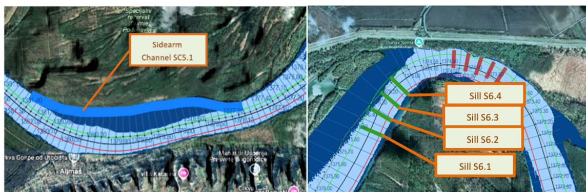
Figure 99 - The locations envisaged for the sidearm channel trenching and construction of the sills on the Staklar section
