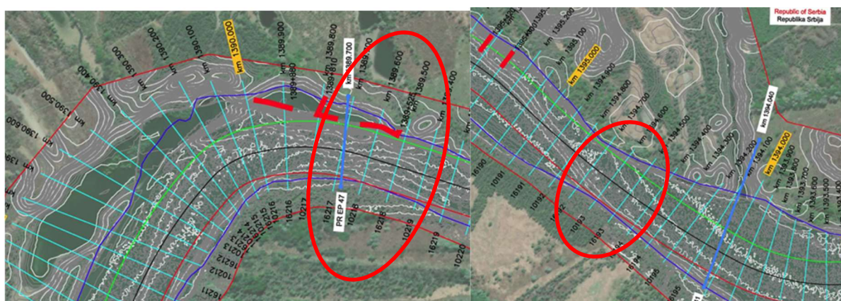
Figure 65 - The contractions in the Čivutski / Židovski rukavac sector on km 1394.6 and 1389.5
