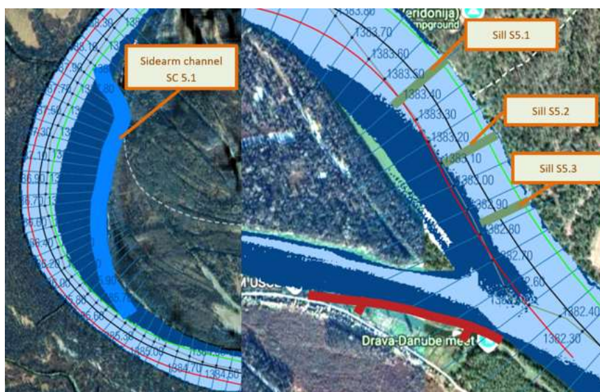
Figure 91 - The map of the structural measures analyzed along the Drava Confluence Sector – Sidearm channel 5.1 and Sills 5.1, 5.2 and 5.3
