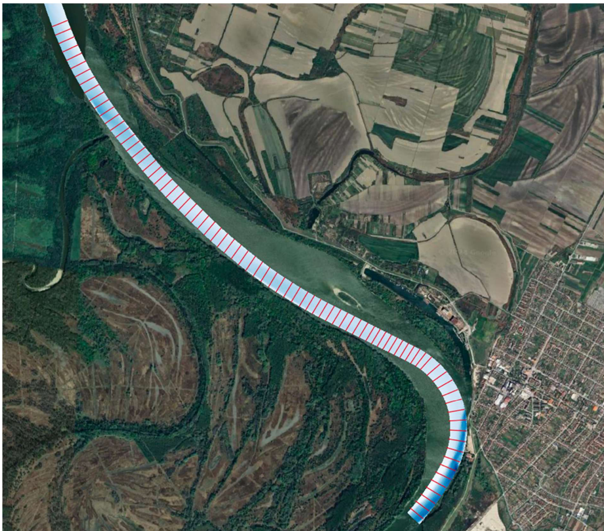
Figure 168: Profiles used in the Apatin sector to determine the longitudinal distribution of minimum depths for Scenario 1 (Different shades of blue indicate depths within the fairway at Q_{94\%} )
