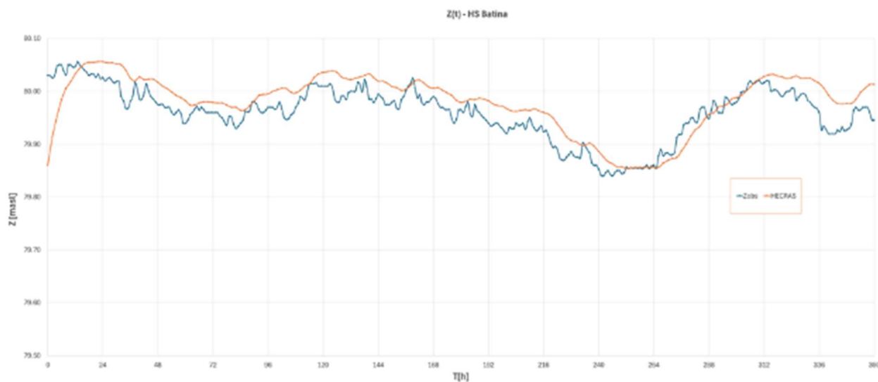
Figure 16: HS Batina (Danube), Comparison between Calculated (red line) and Observed elevations
