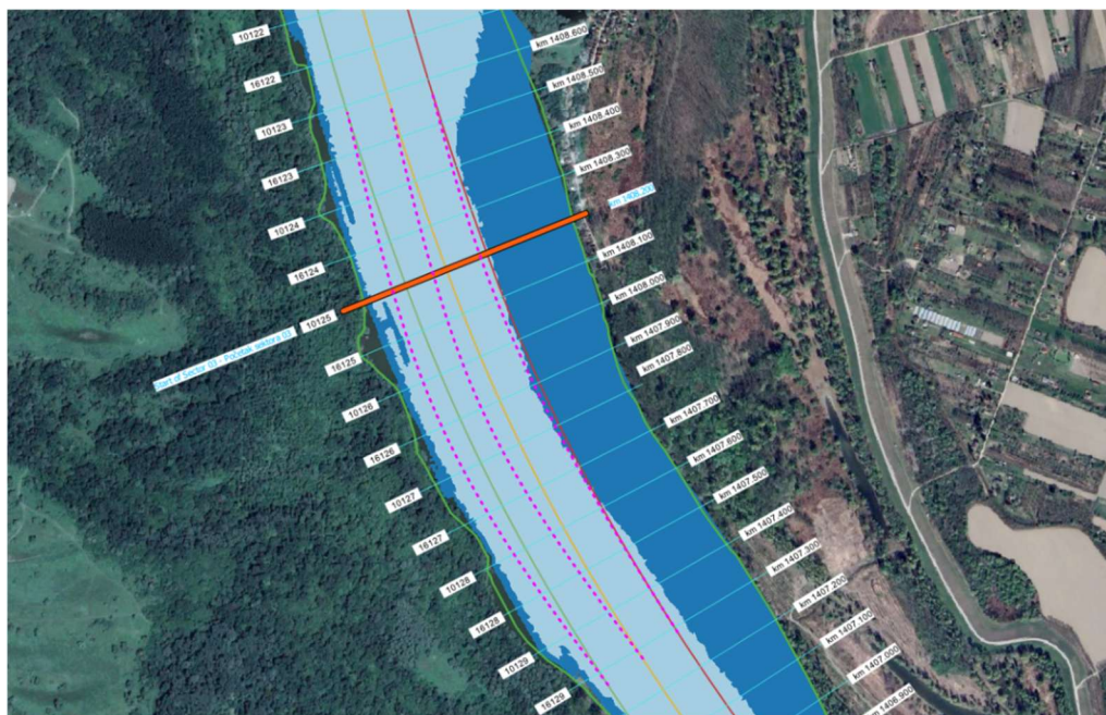
Figure 82. Fairway realignment at the critical section from rkm 1408.200 - 1407.300
